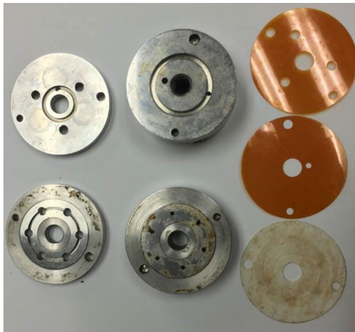
Liquid Contaminated Valve
