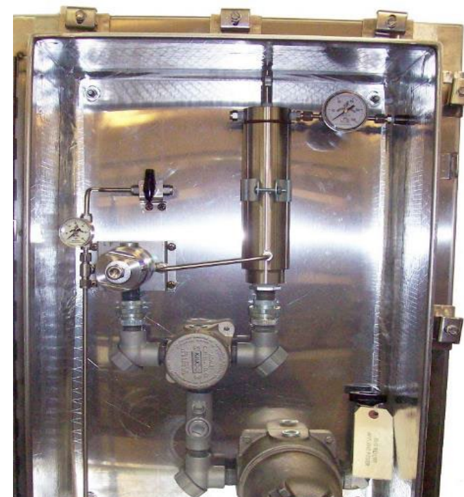
Heated Vaporized Stream SHS
