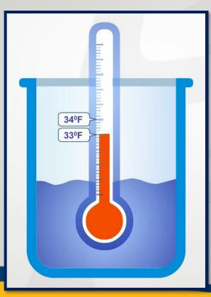
**SENSIBLE HEAT-** The thermal energy absorbed or transmitted by a substance during a change of temperature which is <u>not</u> accompanied by a change of state.
