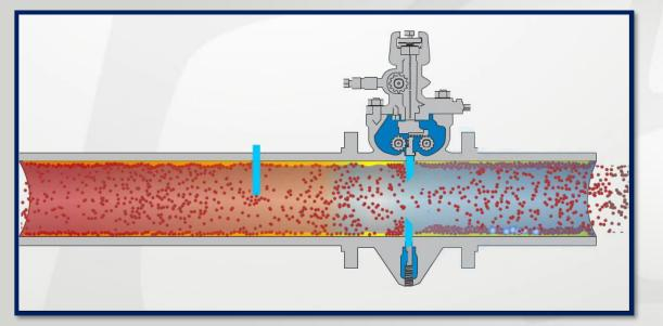
• Cooling that occurs when a highly compressed gas is allowed to expand in such a way that no external work is done.
