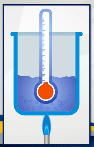
LATENT HEAT OF VAPORIZATION -The heat required to change a liquid to a gas or vapor, without a change of temperature. It is also the heat released in the reverse process.
