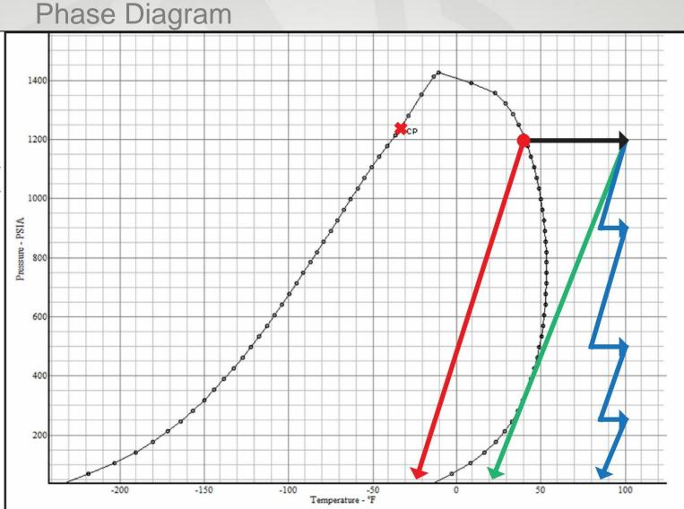
• Valve & regulator freeze-ups are usually caused by Latent Heat of Vaporization, not Joule-Thomson cooling, especially in sample systems.
