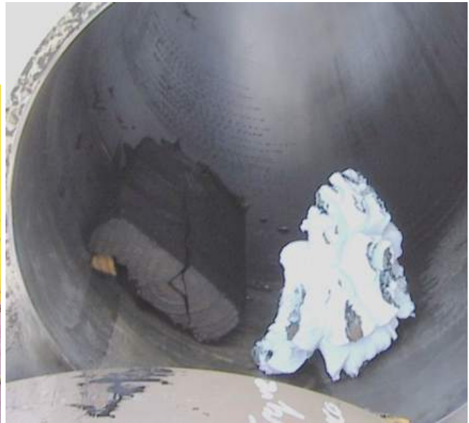
Figure 26 – 12-inch Flow Conditioner Blockage
