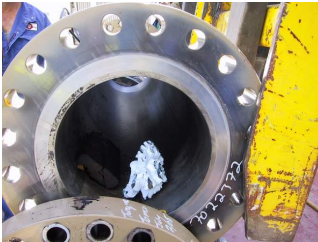
Figure 25 – 12-inch Flow Conditioner Blockage
