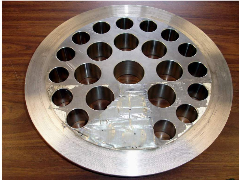
Figure 10 – 3 Holes Blocked Flow Conditioner
