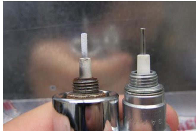
Flame sensor (7.7 mg Si/m 3 , approximately 71 hours, equivalent to 0.5 month of normal operation)
